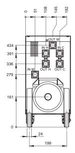
IN H Input hot water circuit OUT H Output hot water circuit
