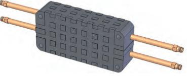
Example for the design of a mould-insert for variothermal control
