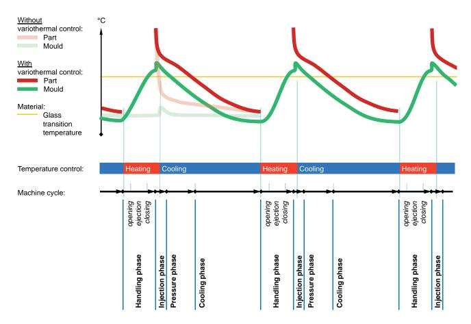
Process procedure in injection moulding with variothermal control
